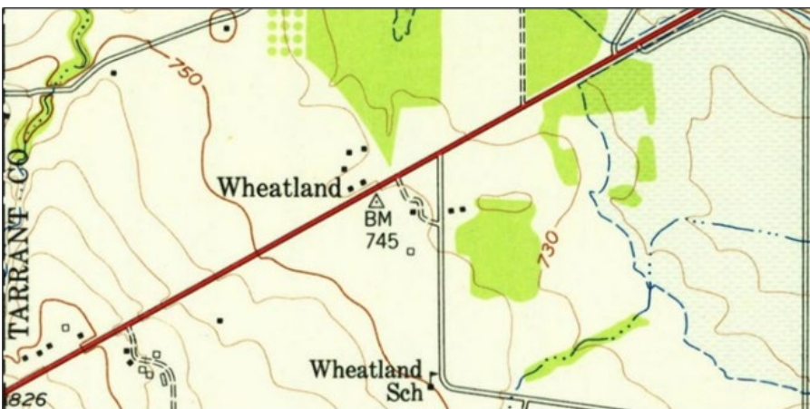
Figure 5-1. Excerpt from a 1955 topographic map of Tarrant County (USGS Cresson Quadrangle, Texas, 1955). Historical topographic maps depict the locations of buildings (as black and white squares and rectangles) and other built resources like roads, dams, and airports. By overlaying topographic maps with current maps with appraisal district data, the locations of potentially extant historical properties can be identified.
